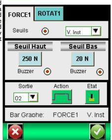
The <u>Centor Star Touch</u> can operate in two different measurement modes: continuous and test. Under continuous mode, the force gauge measure permanently the force but it can't plot the graph or determine specific calculations.
